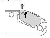
**2** Disconnect the connector of the battery pack and pull the old one out.
